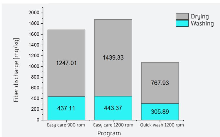
Illustration of the fiber discharge with different washing programs and/or increased spinning speed.
