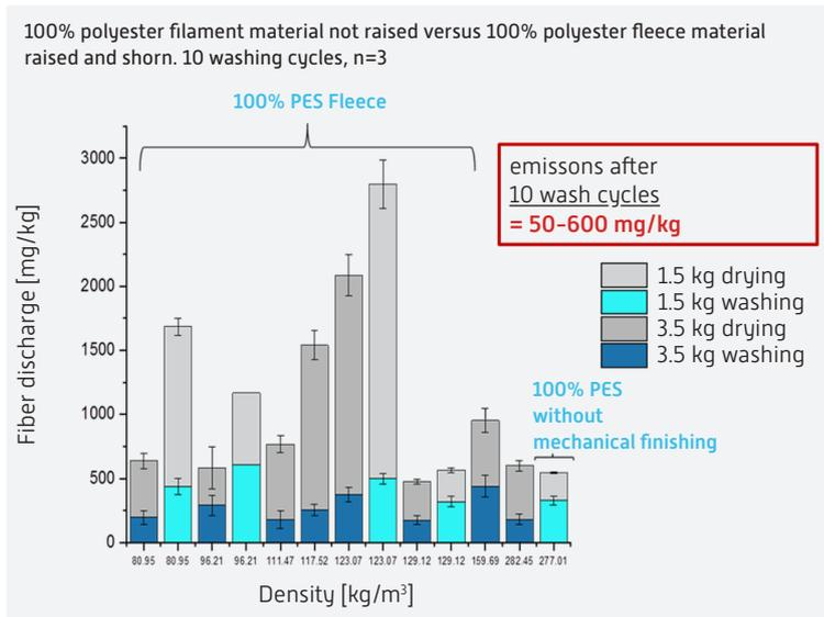
Fiber discharge after 10 household laundry and 10 tumble dryer cycles for 100% PES fleece fabrics with and without mechanical finishes.
