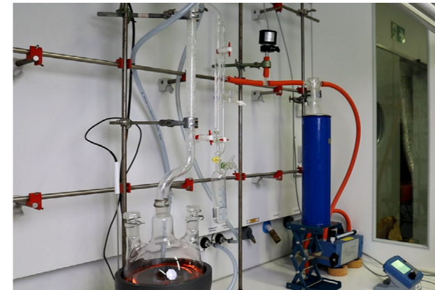
Purification of the condensate by distillation on the laboratory scale.
