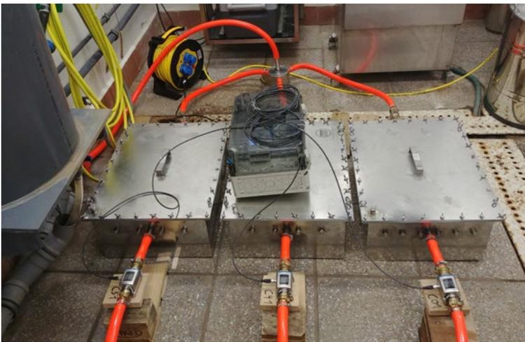
Use of pump-driven sedimentation boxes in a measuring station
