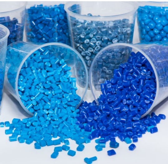
Granules or pellets are easily pourable particles measuring a few millimeters.
