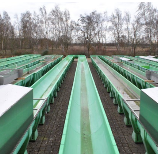
Mesocosms are usually simplified and partially enclosed experimental facilities used to simulate near-natural conditions.
