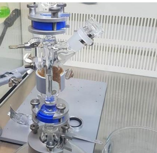
Two-stage filtration apparatus designed to prepare microplastics for analysis.
