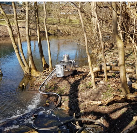
The sampling device „Rocket“ is used to take samples in limnic systems.
