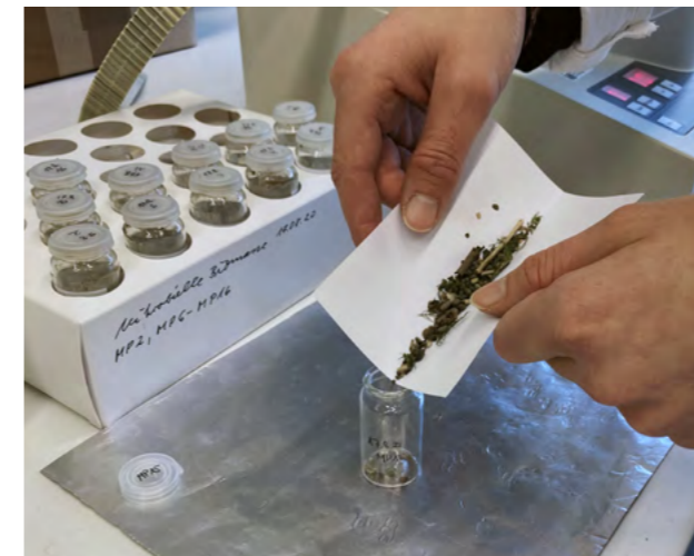
Before determining the microplastic content, the lake sediment is separated into particle size categories.
