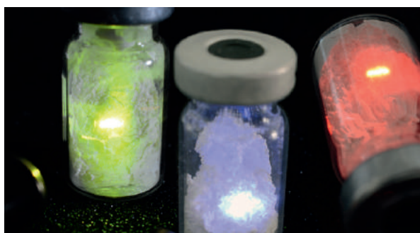
Fluorescent markers should enable improved sorting of plastic packaging.
