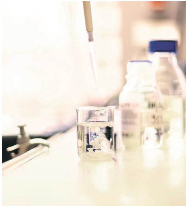
Precipitation of terephthalic acid (TPA) from dissolved PET
