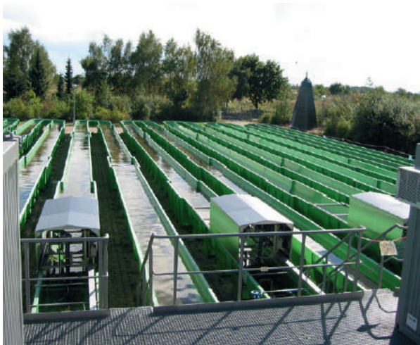
Flow and pond simulation facility of the German Environment Agency in Marienfelde
